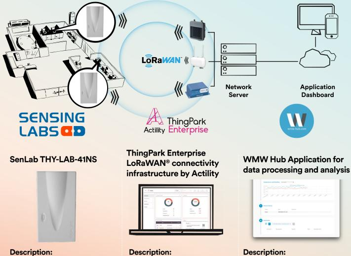
This device offers accuracy of ±0.3°C and ±2% RH maximum (with an operating range of 0 to 100% RH). Designed for indoor use, Senlab™ H has a small casing with a discreet aesthetic that makes it ideal for housing or office.
