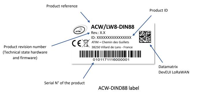
Each product in ATIM's ACW range has a QR Code label visible either on the side or on the front of the product. This QR Code can be easily read with any 2D barcode reader app on your smartphone.
