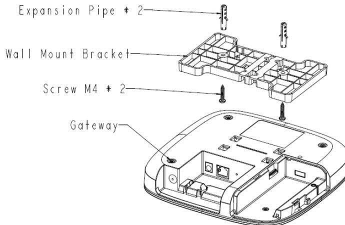
**Figure 4. A Typical Wall or Ceiling Mount Deployment**
