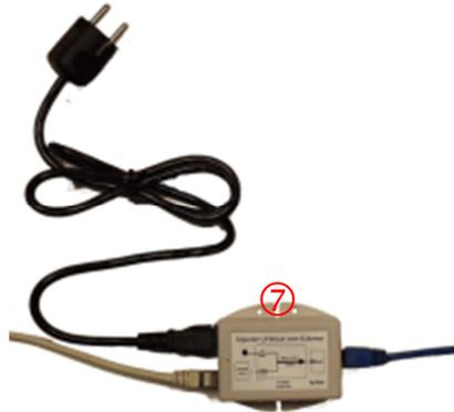
Figure 4 : POE injector (example)
