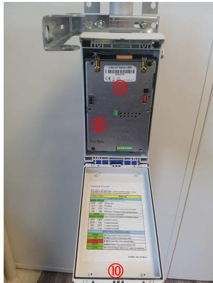
Figure 5 : LoRa IoT Station casing - internal view
