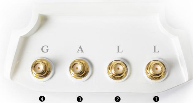
Figure 1.2: Antenna connectors of MX1901/2 Gateway.
