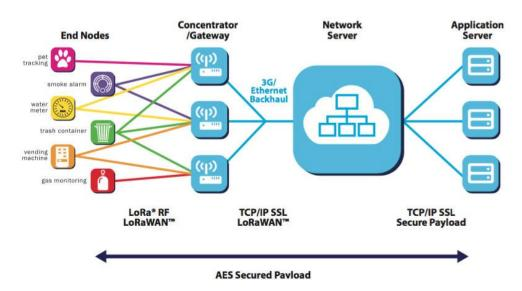
SL101EU temperature and humidity sensor is based on standard LoRaWAN Class A, so you can connect to any LoRaWAN network as below:
