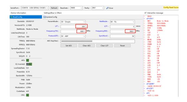
5. Update config, and when configuration update successfully, close the config tool, and local configuration has been finished.
