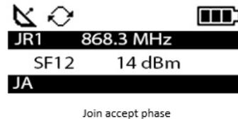
The request are identify «JR» following with a number showing the number of request done. The frequency used for the request is showing after this information.
