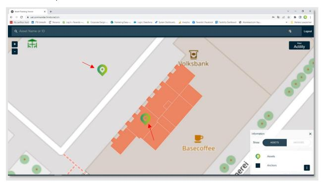
Please note that the update rate of the trackers is set to 60 seconds by default. Meaning that the position of the trackers will be recalculated and updated every 60 seconds.
