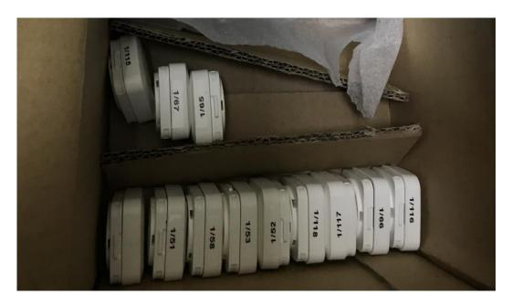
To place the Anchors at the correct position, you need to match the labels on the Anchors with the IDs of the Anchors that you can see in the ATV on your floorplan. Each Anchor has its own predetermined position!
